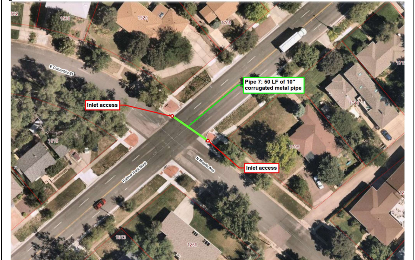
Figure 6: Pipe 7 to be lined on Palmer Park Blvd
