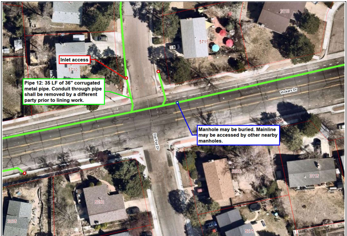
Figure 11: Pipe 12 to be lined on Vickers Dr
